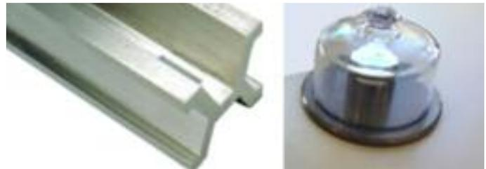
Until 1960, the international length standard was defined by two marks inscribed on a bar of platinum-iridium. In 1960, the meter as an artifact was replaced by a definition of the meter in terms of a constant of nature. Internationally, a meter is now defined as the length of path traveled by light in a vacuum during a time interval of  $1/299,792,458$  of a second.
